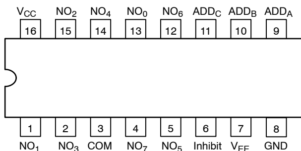
Figure 1. Pin Connection (Top View)
